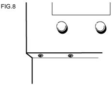
3 Tilt the bottom of the fascia panel out over. Withdraw the fascia panel by moving it down over to disengage it from the top fixing lugs.
